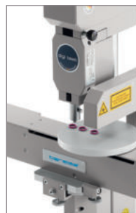
Laser-controlled positioning of O-rings
